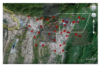
Trillium 40, three component sensors. The network spans an area of approximately 1900 km<sup>2</sup> covering the most of VC block area in order to ensure complete subsurface coverage (Fig.2). Recording began on 19<sup>th</sup> of November 2009 and completed on the 23<sup>rd</sup> of February 2010.
